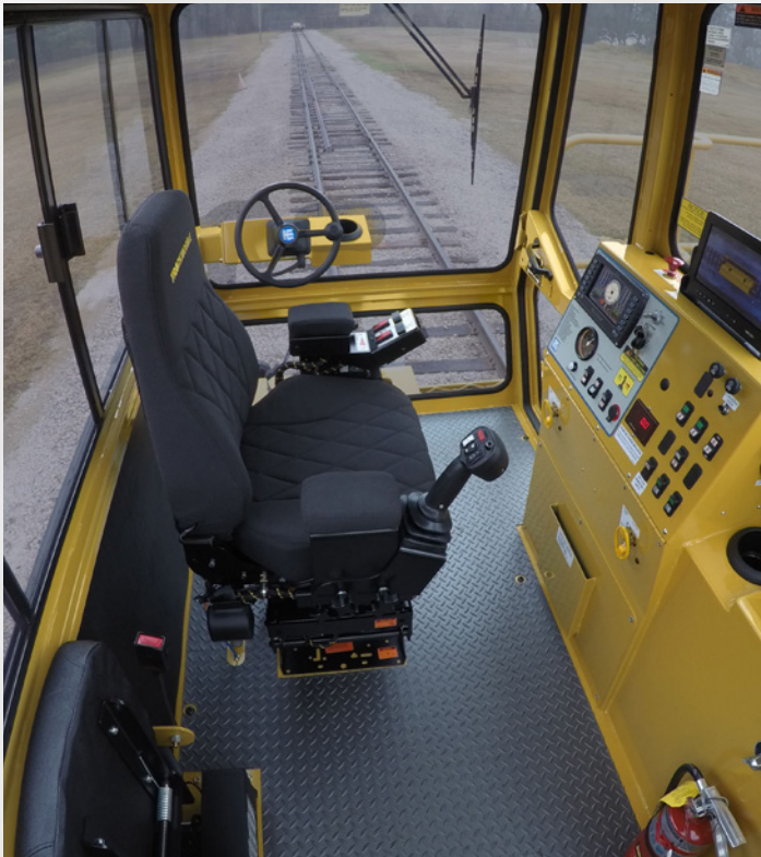
Hercules control panel and operational controls.
